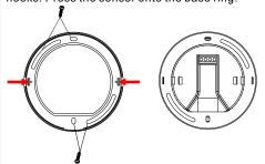
Note: The mounting clips indicated by the arrows represent the direction of the longer ultrasonic range shown in the Detection Area diagram.
